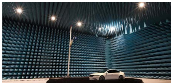
Figure 36.5: An anechoic chamber for radio frequency. In such an electromagnetically quiet chamber, interference from other RF equipment is minimized (courtesy of Panasonic).
